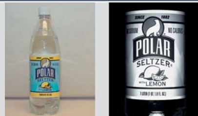
Object: Labeled bottle. Image captured with Area Array. Inspect for label presence or absence, correct label and proper orientation.
