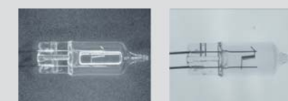
Object: Miniature lamp. Image captured with Backlight. Inspecting integrity of lamp filament.
